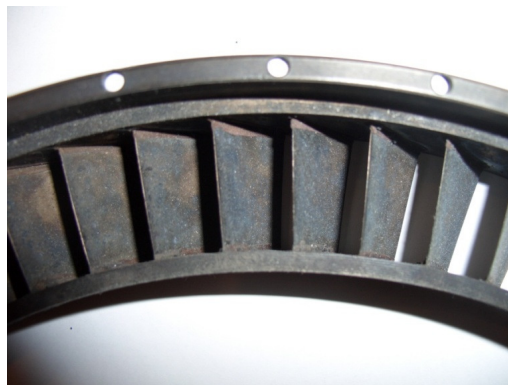
Fig. 1. Stator vanes of GTE-TV2-117A
