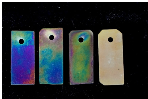
Fig. 4. Samples after testing: (149-150-151-basic) 800 °C
