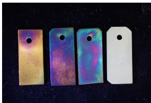
Fig. 3. Samples after testing: (149-150-151-basic), 750 °C
